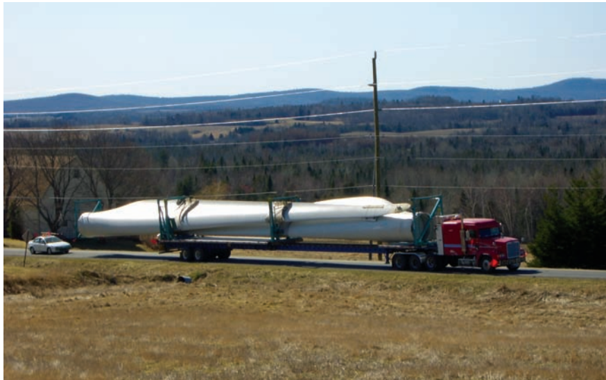
A stretched-out tractor trailer hauls two windmill blades to the job site.
