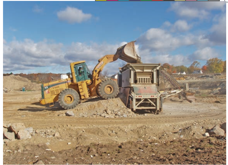
Nationwide Rock Rock and Recycling Corp.'s Kawasaki loads rock into a Lippman 30 X 48 jaw crusher.
