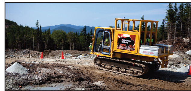
Crew access to a pioneered area is assured with the Komatsu Crew Transport.
