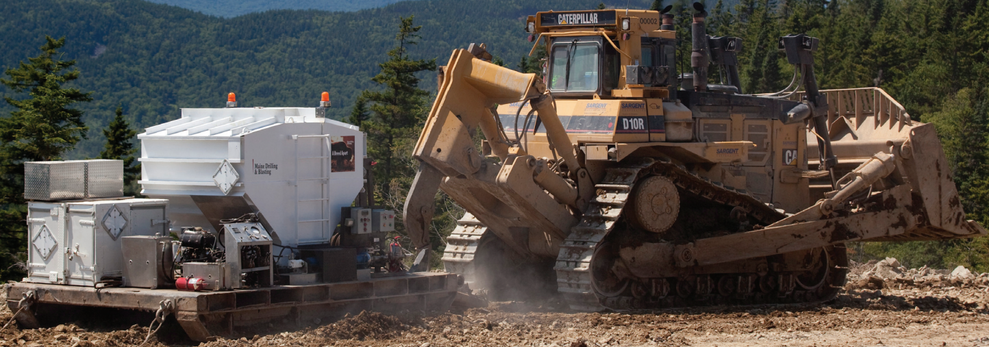
The Bulk Skid™ being dragged by a D-8 class dozer, so 10,000-pounds of bulk can be pumped to multiple holes in an area where there are no roads.
