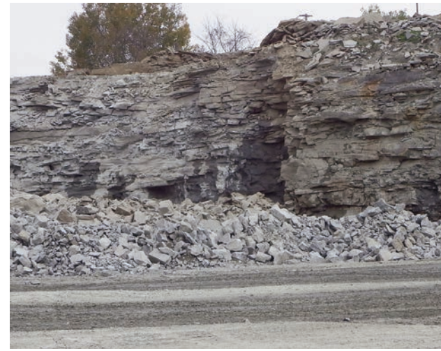
Drilling and blasting in this kind of formation, makes successful blasting more difficult than in more solid geology.
